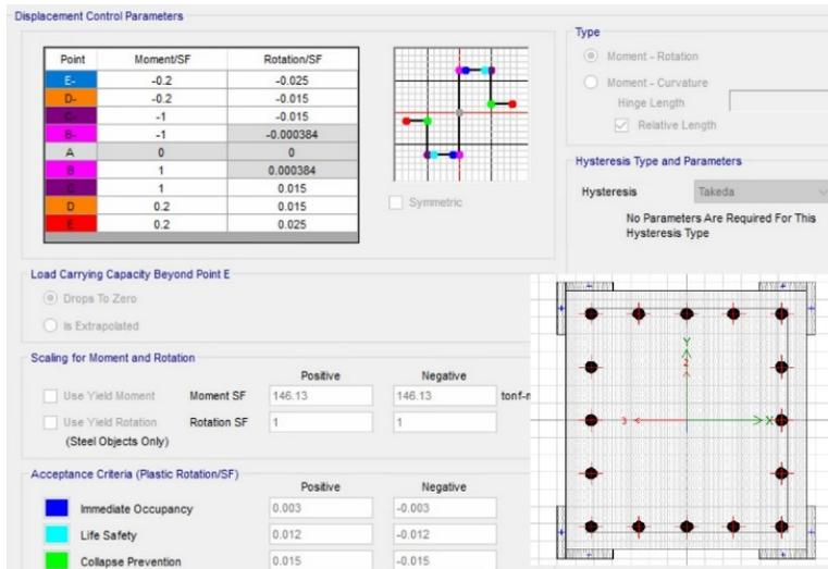
Image 5. Plastic hinge parameters of a column of the SFRS
