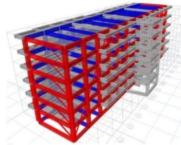
Image 2 Analysis models for the project. Complete system, (in red interior) and OMF (in blue exterior) as a back-up system
