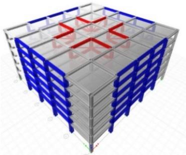
Image 1 Schematic representation of a complete model. SFRS as SCBF (in red interior) and OMF (in blue exterior) as a back-up system
