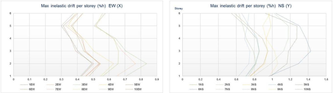
Image 7. Max inelastic drift short (Y) side (bottom), long side (X) (top).
