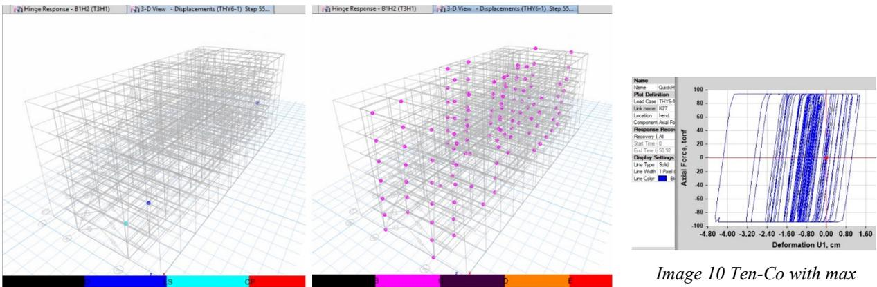
Image 9 Hinge states (left) and Hinge status (right) during 6NS ground motion
