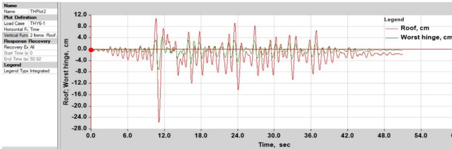
Image 8 Displacements at the roof and storey 2, ground motion 6NS (Y)
